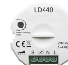
FD-LD440 Dimmer for LED lamp Power: 440W 230V 50/60 Hz Installed in the mounting box behind the push button. Dimensions: 56 x 22 mm Units: 1
